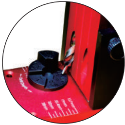
Drill depth turret for setting up
